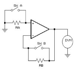
$V_{supply} = +/- 15$  VDC. Pick R<sub>A</sub> and R<sub>B</sub> somewhere between 2M and 10M  $\Omega$ . They need NOT be matched, or even equal.
